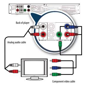
3 Connect an analog audio cable to the AUDIO OUT jacks on the back of your DVD player and to the audio in jacks on the TV.
